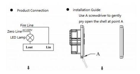
◆According to the product connection diagram, LED load and power supply must be exactly
